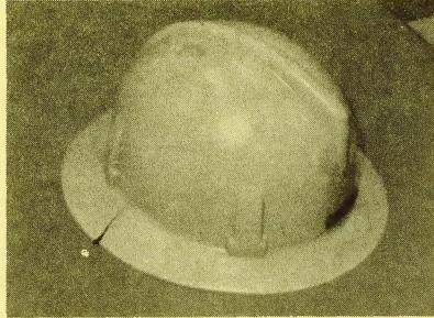
Employees using safety hats should take a good look for cracks or other damages. Old safety hats, with cracks such as the one shown here, don't give the adequate protection needed on the job. Owners of damaged helmets should request new ones through their respective departments.
